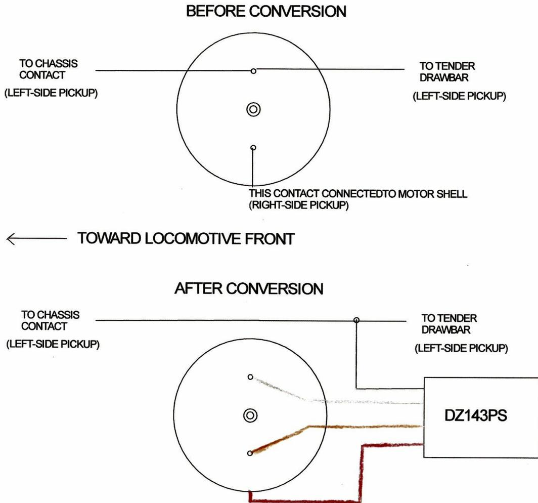
LEFT-SIDE WIRES REMOVED FROM MOTOR CONTACT AND CONNECTED TO DZ143PS BLACK WIRE. MOTOR SHELL DISCONNECTED FROM MOTOR CONTACT AND CONNECTED TO DZ143PS RED WIRE. DZ143PS ORANGE WIRE CONNECTED TO RIGHT-SIDE MOTOR CONTACT. DZ143PS GRAY WIRE CONNECTED TO LEFT-SIDE MOTOR CONTACT.
