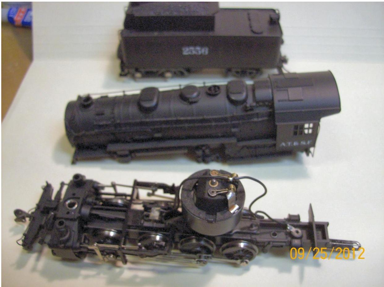
A flash-why not convert it to DCC? With the multimeter and the test power, I discovered the electrical layout. The manufacturer's specs said it was rated for 12VDC at 0.4A maximum. There would be room in the firebox for a z-scale DCC decoder.
